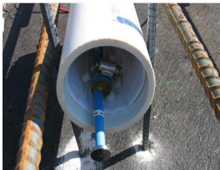
现场温湿度耦合条件下水泥混凝土线膨胀系数测试体系 Cement Concrete Coefficient of Linear Expansion Detection System
