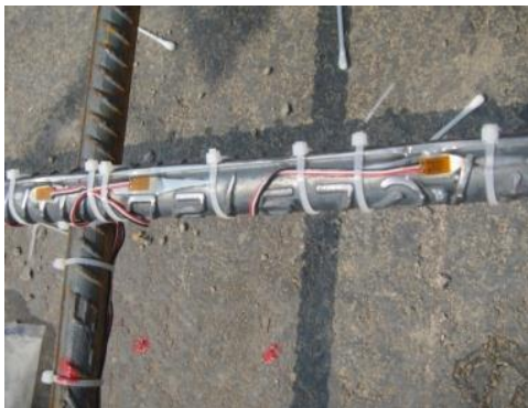
现场温湿度耦合条件下水泥混凝土线膨胀系数测试体系 Cement Concrete Coefficient of Linear Expansion Detection System
