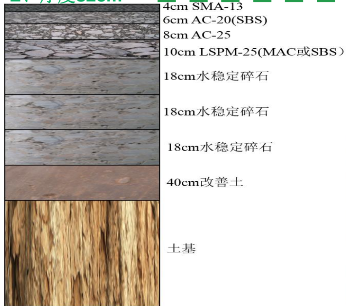
组合式基层耐久路面结构 Combined Based
