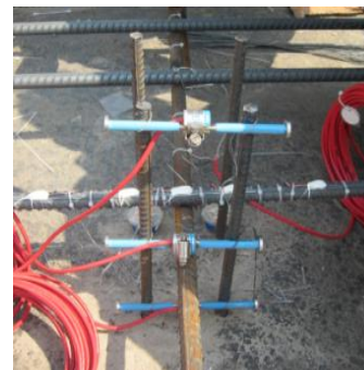
现场温湿度耦合条件下水泥混凝土线膨胀系数测试体系 Cement Concrete Coefficient of Linear Expansion Detection System
