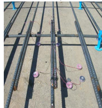
现场温湿度耦合条件下水泥混凝土线膨胀系数测试体系 Cement Concrete Coefficient of Linear Expansion Detection System
